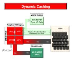
Figure 1. Hybrid Storage Pool architecture
